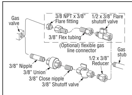
These fireplaces are equipped with a gas flex line for use (where permitted) in connecting the unit to the gas line. A gas flex line is provided to aid in attaching the direct-vent fireplace to the gas supply. The gas flex line can only be used where local codes permit. The flex line is rated for both natural and propane gas. A manual shut off valve is also provided with the flex line.
