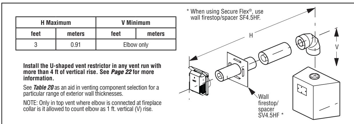
**Table 23 - Top Vent—One 90° Elbow, Elbow Connection NOT at Fireplace**
