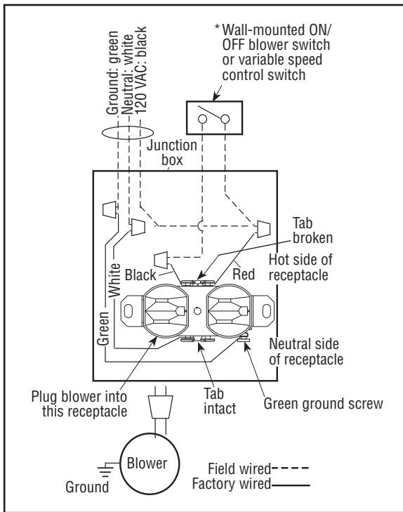
**Figure 33 - Wiring Diagram—Millivolt Gas Valves**
