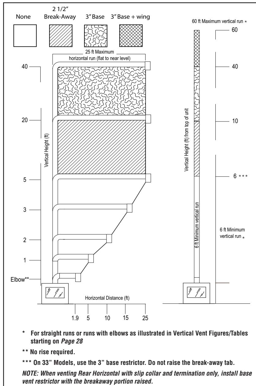
**Figure 13 - Vent restrictor installation, Top vent**
