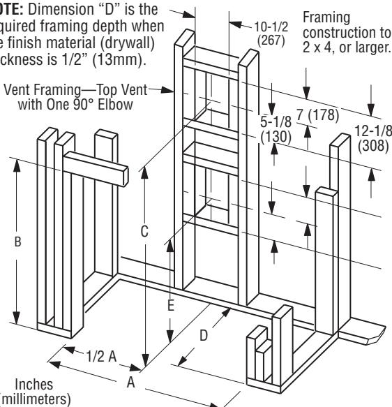
**Table 11 - Fireplace Framing Specifications—Corner Installation with Horizontal Termination**
