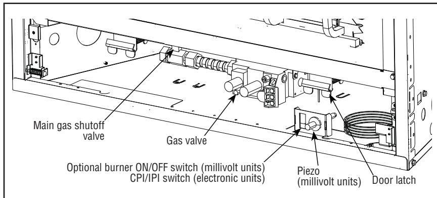
**Figure 35 - Gas Line Connection**
