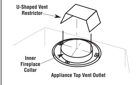
**Figure 14 - Vent restrictor installation, Rear vent**
