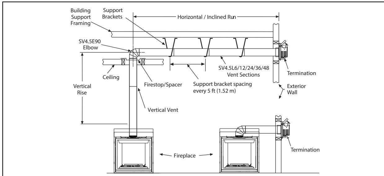
1. **Analyze the vent route and determine the number of vent sections and elbows required**—See **Effective Vent Length on Page 24** for more information. Plan the venting so that a joint does not occur in the ceiling or roof joists. Allow for elbows (**Figure 18**). Maintain the minimum clearances for combustibles (**Page 14**).
