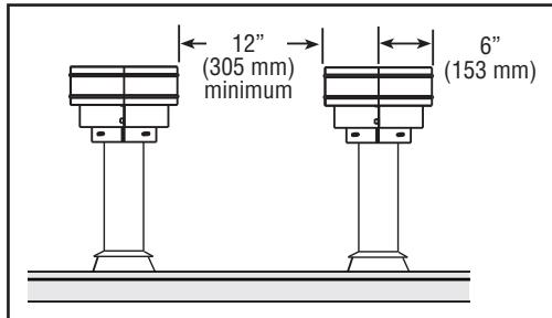
Terminate single vent caps relative to building components according to **Table 6** and **Figure 4**.
