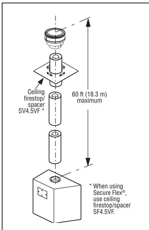
Install the U-shaped vent restrictor in any vent run with more than 6 ft of vertical rise. See [Page 22](#) for more information.
