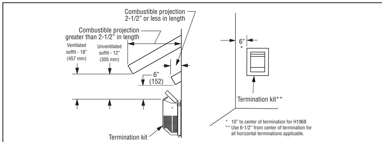
**Table 7 - Horizontal vent termination clearances for buildings with combustible and noncombustible exteriors**
