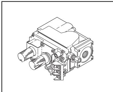
**Figure 2 - Electronic Gas Valves**
