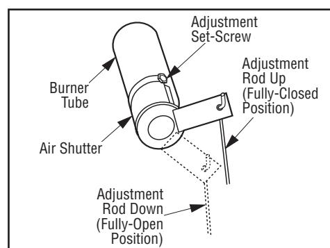
1. Move the adjustment rod down to increase air flow and up to decrease it. The rod is located in the lower control compartment. Position the air shutter to the factory setting (**Table 29**).
