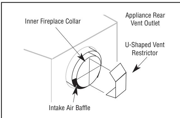
**Figure 15 - Vent restrictor assembly**
