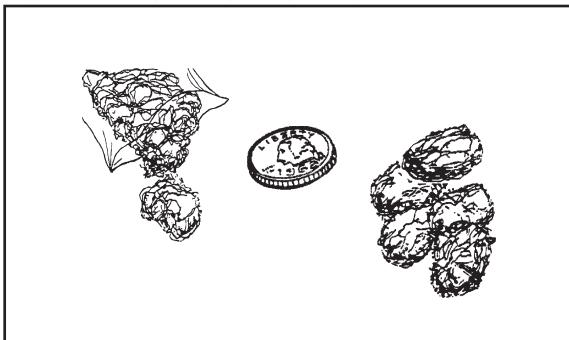
5. In traditional units, position the separated glowing embers over the small holes on the burner surface ([Figure 49](#)). Do NOT cover the large burner slots.
