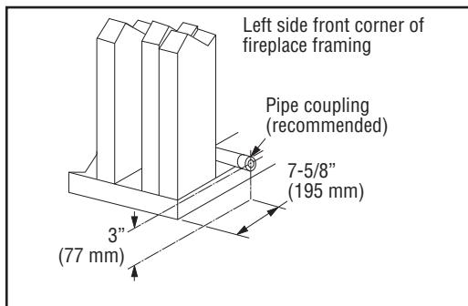
**Figure 10a - Routing the Gas Line - 33" Model**
