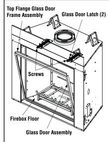
Figure 62—Glass Door Assembly Removal/Installation
