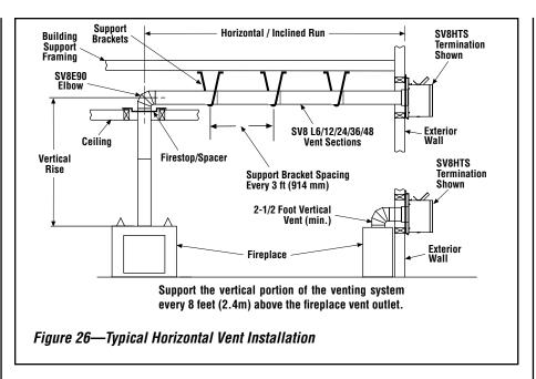
Push the vent component against the collar until it fully engages, then twist the component clockwise, running the dimples down and along the incline channels until they seat at the end of the channels. The unitized design of the **Secure Vent** components will engage and seal both the inner and outer pipe elements with the same procedure. Sealant and securing screws are not required.
