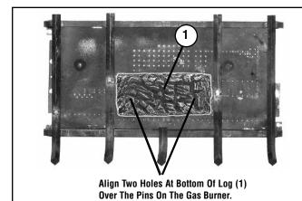
Figure 66 - Placing Log 1
