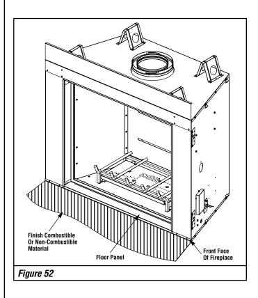
**NOTE:** A finish trim piece is shipped with your fireplace to extend the base 1/2" to be flush with the finish flanges on the side of the fireplace. This filler is shipped on top of the fireplace wrapped in foam. If desired this piece can be placed on the base of the fireplace. It is secured with bend tabs on either side. Lay the extension in front of the base then secure by bending tabs on each side over to secure to the base. While this piece is provided it is not required.
