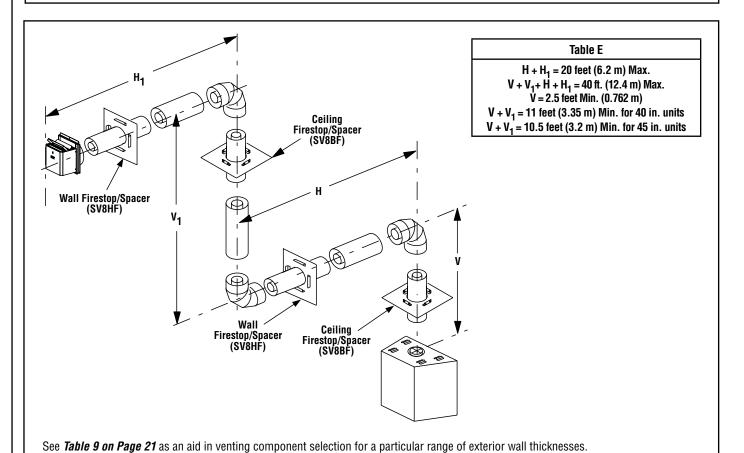
Figure 31—Top Vent—Three 90 Degree Elbows
