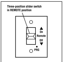
Figure 34—Receiver (Wall Switch)
