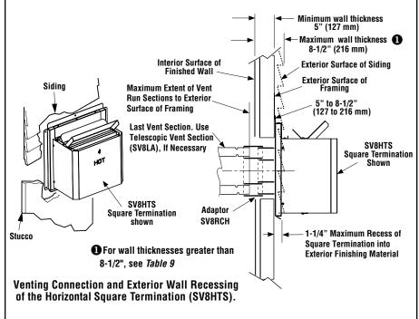
Figure 28—Wall Thickness and Horizontal Termination Requirements
