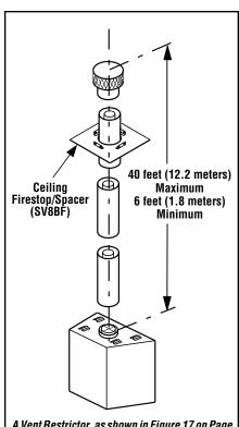
A Vent Restrictor, as shown in Figure 17 on Page 12, may need to be used in this application
