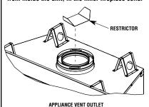
Figure 14—Vent Restrictor Installation
