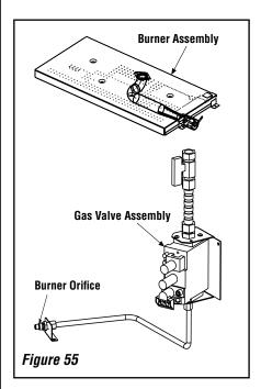
**Step 5.** Remove the control compartment access door and gasket by removing the twelve (12) screws securing it, and set it aside for later reinstallation. The gas valve can be accessed through the opening, or the complete assembly can be removed by sliding the assembly to the right.
