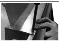
Step 2. Affix shield with 5/16" hex screws into front standoff.
