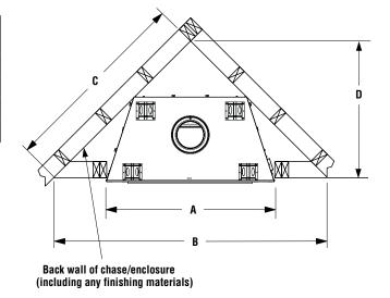
Figure 12—Corner Framing with Square Termination (SV8HTS)
