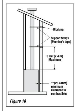
One method of support is by utilizing field provided support straps (conventional plumber's tape). Secure the plumber's tape to the framing members with nails or screws. Strap the tape around the vent, securing the ends of the tape to the framing. If desired, sheet metal screws  $\#6 \times 1/2"$  length may be used to secure the support straps to the vent pipe. See *Figure 18 on Page 16*.
