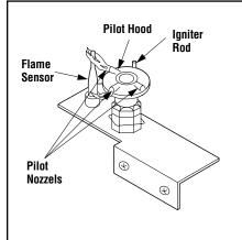
Figure 74—Pilot Assembly— Proper Pilot Flame Appearance
