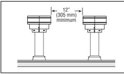
Terminate single vent caps relative to building components according to Table 6 and Figure 4.
