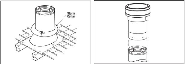
**12. Install the vertical termination**—Extend the vent sections to the correct height (*Table 6*). The SV4.5CGV-1 Vertical Termination (*Figure 21*) installs in the exact same fashion as any other Secure Vent<sup>®</sup> section.
