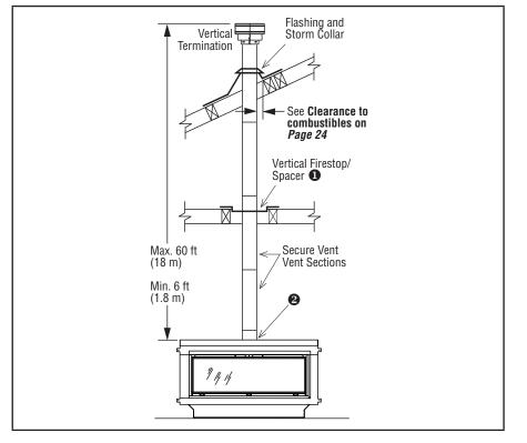
Install the U-shaped vent restrictor in any vent run with more than 6 ft of vertical rise. See Page 21 for more information.
