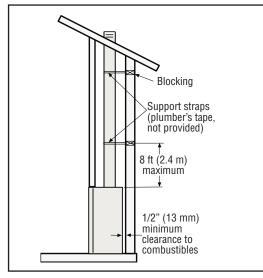
Figure 19 - Supporting the Vertical Vent Run
