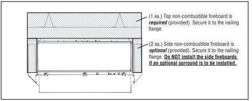
**NOTE:** The provided non-combustible fiberboard may be skim coated as a finish material, however, other types of non-combustible board may provide a more durable surface.
