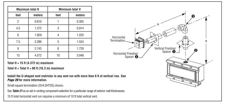
• Vertical firestop/spacer must be used anywhere vent pipe passes through a combustible floor or ceiling. Horizontal firestop/spacer must be used anywhere vent pipe passes through a combustible wall.
